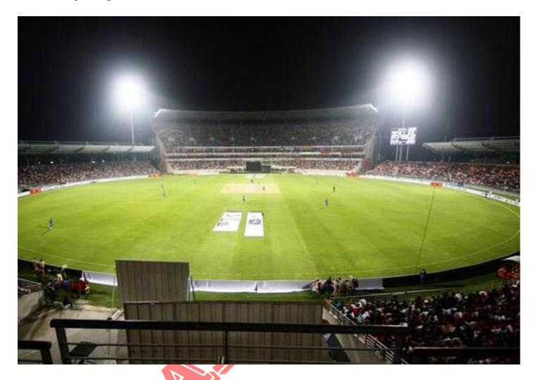
Generally, a brightness level ranging between 250 and 350 lux would be enough for players and spectators in normal cricket games. However, this isn't quite there when it comes to professional matches, which would need a brightness level ranging between 500 and 750 lux. The brightness level should be much higher, somewhere in the range of 1500 to 2500 lux, if the matches are to be broadcasted live.
